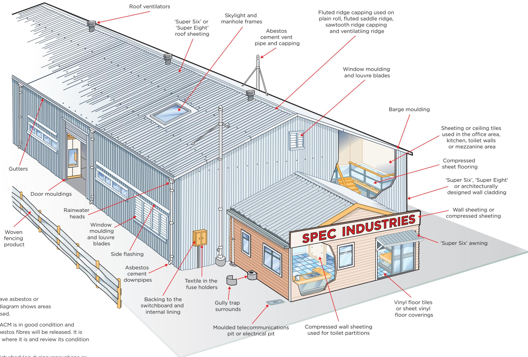
Buildings constructed before 2000 may have asbestos or asbestos-containing material (ACM). The diagram shows areas where asbestos or ACM were commonly used.
